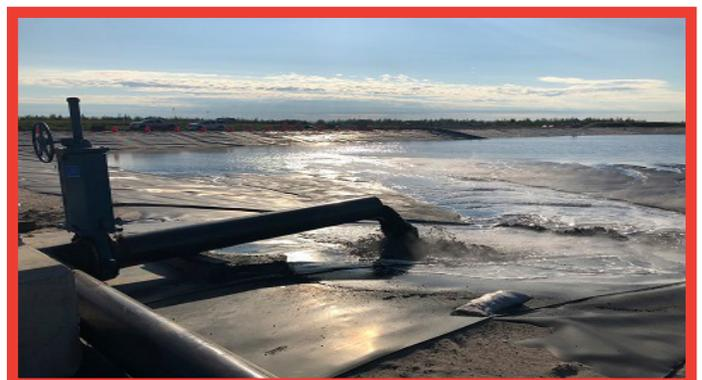
*Tailings flowing into the filtration cell.*
